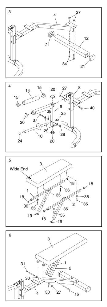
With the wide end of the Seat (5) positioned as shown, attach the Seat to the brackets on the Bench Frame (4) using four M6 x 16mm Screws (32).
